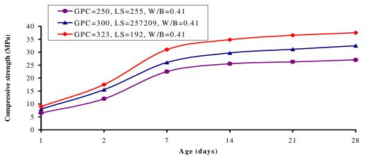
Fig. 6: Compressive Strength of SCC Containing Milled Limestone and Different Cement Contents
