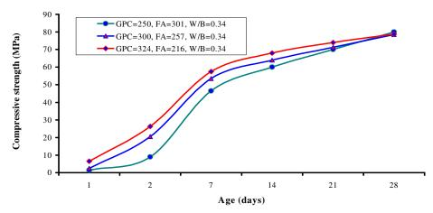
Fig. 5: Compressive Strength of SCC Containing Fly Ash and Different Cement Contents
