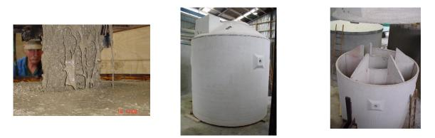
Fig. 7: Pour of SCC; Septic Tank with the Roof and "Wing-Wall" Insert
