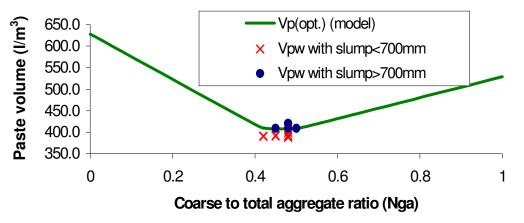
Fig. 3: Minimum Computed and Tested Paste Volumes and Different Coarse to Total Aggregate Ratios
