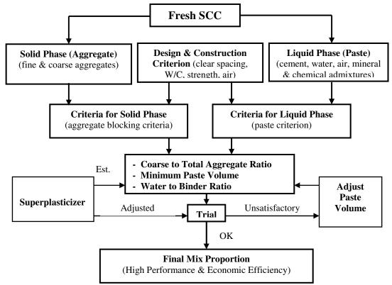
Fig. 1 Mix Design Procedure Flow Chart
